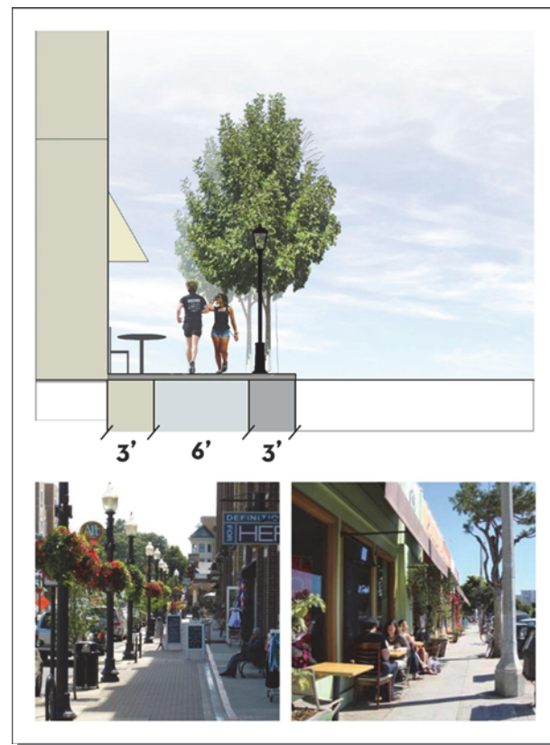
Figure E2 – Typical 10' - 14' Pedestrian Zone
