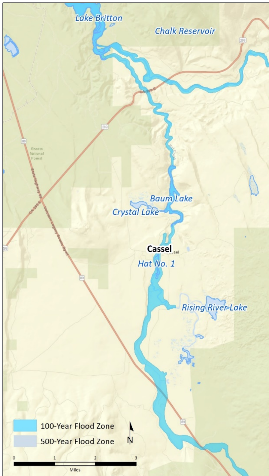
Figure 79. Flooding hazards associated with Hat Creek threaten Highways 89 and 299 near Cassel.
