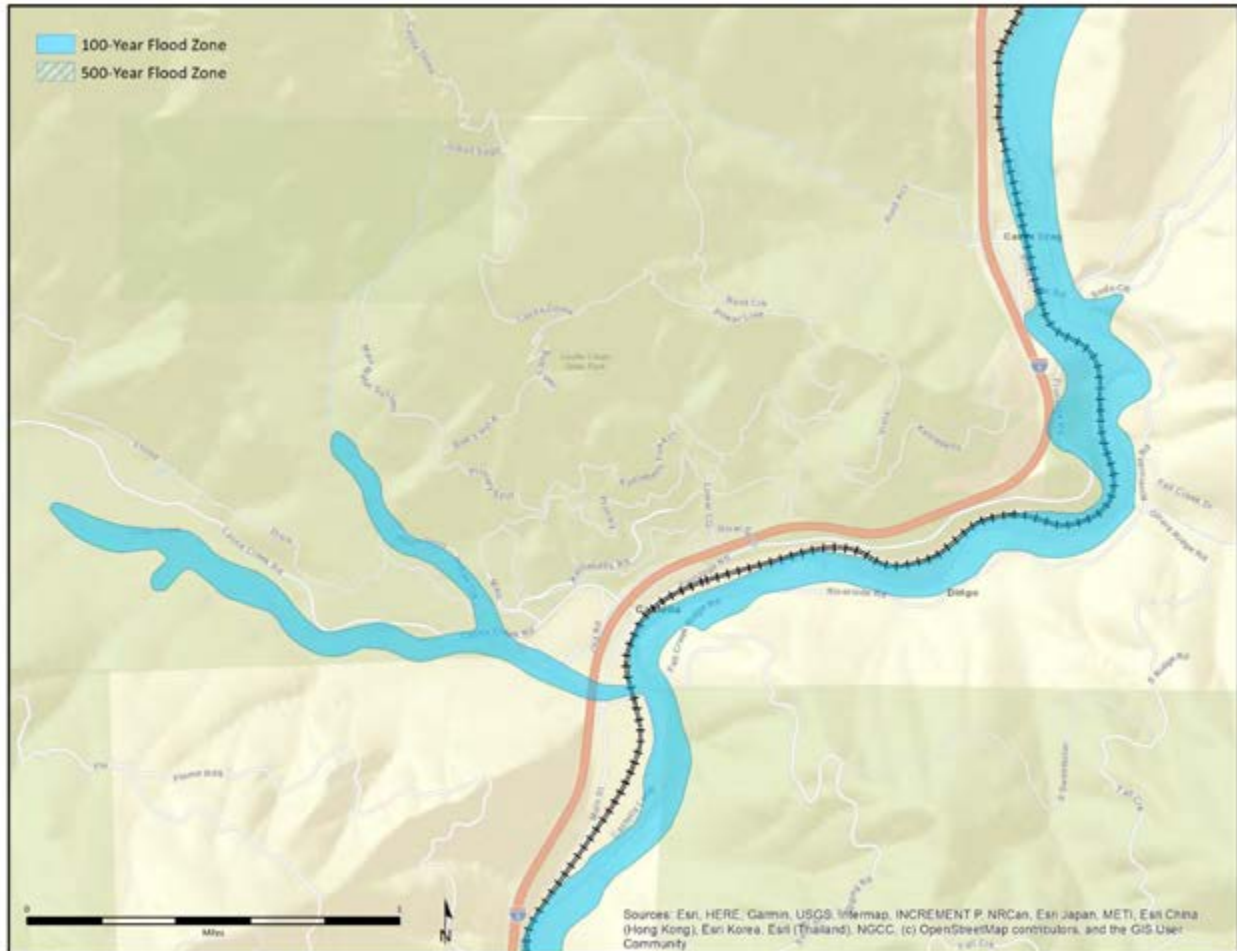
Figure 73. Flooding exposure of the Union Pacific Railroad in the Sacramento River Canyon, near Castle Crag State Park.
