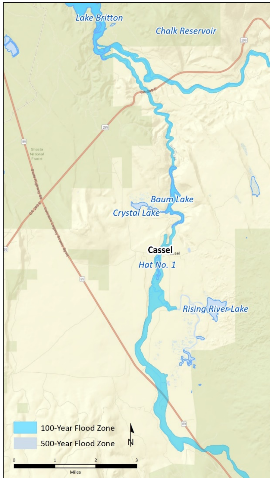
Figure 78. Flooding hazards associated with Hat Creek threaten Highways 89 and 299 near Cassel.
